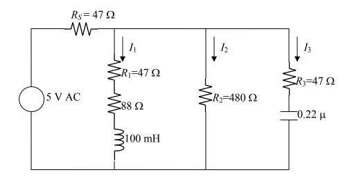
Figure 2 Parallel AC circuit.
