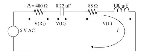
Figure 1 Series AC circuit.
