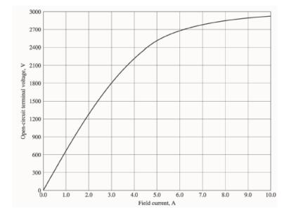
(a) If the no-load terminal voltage is 2300 V, the required field current can be read directly from the open-circuit characteristic. It is 4.25 A.
