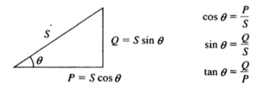
The quantity  $\cos \theta$  is usually known as the *power factor* of a load. The power factor is defined as the fraction of the apparent power S that is actually supplying real power to a load. Thus,
