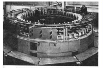
Stator of a 190-MVA three-phase 12-kV 375-r/min hydroelectric generator. The conductors have hollow passages through which cooling water is circulated. (Brown Boveri Corporation.)
