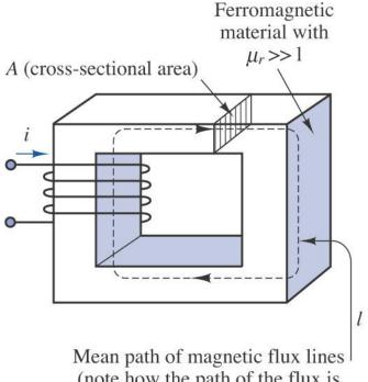
(note how the path of the flux is enclosed within the magnetic structure) Copyright © The McGraw-Hill Companies, Inc. Permission required for reproduction or display.
