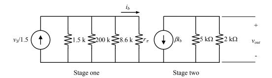
Figure 3: Small-signal circuit of the BJT amplifier.
