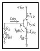
$R_B = R_1 / R_2 = 9.982 \text{ k}\Omega$  $V_{BB} = \frac{R_2}{R_1 + R_2} V_{CC} = 15 \frac{11.7}{11.7 + 68} = 2.202 \text{ V}$
