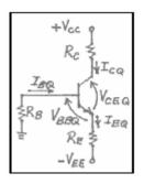
$-V_{EE} + I_B R_B + V_{BE} + I_E R_E = 0$   $I_B = \frac{V_{EE} - V_{BE}}{R_B + (\beta + 1)R_E} = \frac{4 - 0.7}{100000 + 101 \times 3000} = 8.189 \ \mu\text{A}$   $I_C = 100 \times 8.189 \ \mu\text{A} = 818.9 \ \text{mA}$   $I_E = 101 \times 8.189 \ \mu\text{A} = 827 \ \text{mA}$
