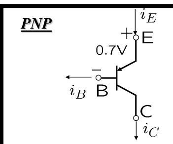
Equivalent Circuit of the PNP BJT in the ACTIVE mode E $I_{S/\beta}$   $\beta I_B$ C
