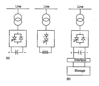
Shunt-connected Controllers: (a) Static Synchronous Compensator (STATCOM) based on voltage-sourced and current-sourced converters; (b) STATCOM with storage, i.e., Battery Energy Storage System (BESS) Superconducting Magnet Energy Storage and large dc capacitor; (c) Static VAR Compensator(SVC), Static VAR Generator (SVG), Static VAR System (SVS), Thyristor-Controlled Reactor (TCR), Thyristor-Switched Capacitor (TSC), and Thyristor-Switched Reactor (TSR); (d) Thyristor-Controlled Braking Resistor.
