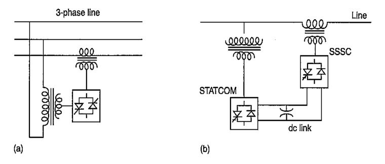
Figure 1.7 (a) Thyristor-Controlled Phase-Shifting Transformer (TCPST) or Thyristor-Controlled Phase Angle Regulator (TCPR); (b) Unified Power Flow Controller UPFC).
