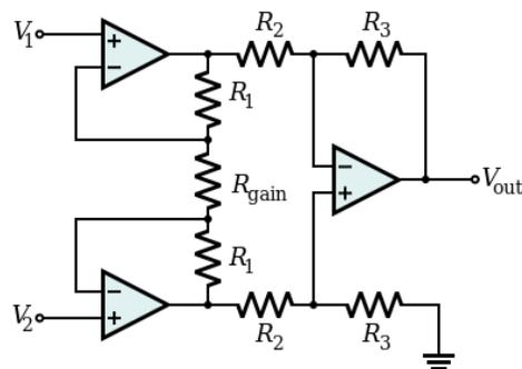
The above device was chosen because it can extract a very small signal difference and attenuates noise resulting from electromagnetic interference. However, something called a motion artifact can still occur due to relative motion between electrodes and the tissue. The frequencies of the motion artifact are usually at the low end of the electromagnetic spectrum. Accordingly a filter (specify) is needed.
