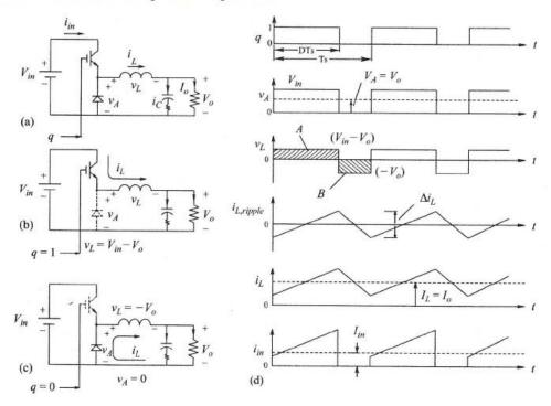
Question 4: Consider a boost converter, the inductor current has  $\Delta i = 2$  A,  $V_{in} = 5$  V,  $V_{o} = 12$  V,  $P_{o} = 11$  W,  $f_{s} = 200$  kHz. Calculate L and values of the generated signal forms.
