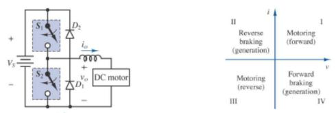
For the Buck circuit ( $S_1$  and  $D_1$ ), determine the duty cycle and turn-on time in the motoring mode if n = 500 r/min, and  $i_0 = 90$  A. Assume  $V_s = 120$  V,  $E_a = 0.1$  n,  $R_a = 0.2$  Ohm,  $f_s = 300$  Hz.
