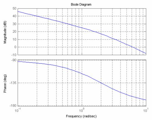
2 Determine the phase margin of the uncompensated system ensure 5 degree addition phase lag
