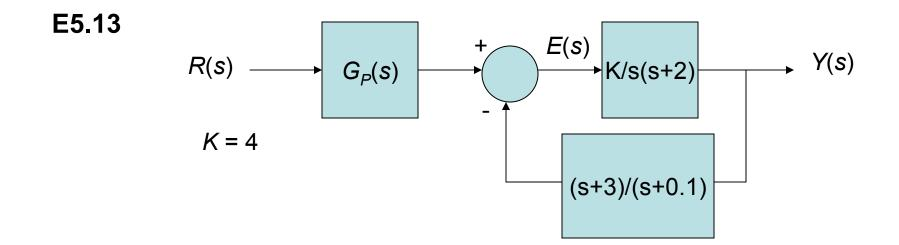
a) The tracking error is given by : E(s) = [1 - T(s)]R(s) (Read Section 5.8) The steady - state tracking error with R(s) = 1/s is  $e_{ss} = \lim_{s \to 0} s[1 - T(s)]R(s) = \lim_{s \to 0} [1 - T(s)] = 1 - T(0)$ The closed - loop transfer function is
