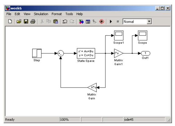
$$A = \begin{bmatrix} 0 & 1 & 0 \\ 0 & -1 & 1 \\ 0 & 0 & -5 \end{bmatrix}, B = \begin{bmatrix} 0 \\ 0 \\ 200 \end{bmatrix}, C = \begin{bmatrix} 1 & 0 & 0 \end{bmatrix}; D = \begin{bmatrix} 0 \end{bmatrix};$$
