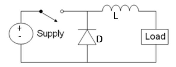
When the switch is closed, the voltage across the inductor is VL = Vi - Vo. The current through inductor linearly rises. The diode does not allow current to flow through it, since it is reverse-biased by voltage V.
