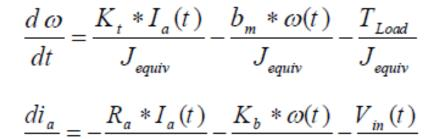
$$\begin{bmatrix} I_{a} \\ \dot{\omega} \end{bmatrix} = \begin{bmatrix} -\frac{R_{a}}{L_{a}} & -\frac{K_{b}}{L_{a}} \\ \frac{K_{t}}{J_{equi}} & -\frac{K_{f}}{J_{equi}} \end{bmatrix} \begin{bmatrix} I_{a} \\ \dot{\omega} \end{bmatrix} + \begin{bmatrix} \frac{1}{L_{a}} & 0 \\ 0 & -\frac{1}{J_{equi}} \end{bmatrix} \begin{bmatrix} V_{in} \\ T_{load} \end{bmatrix}$$
