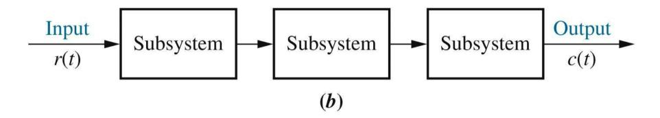
Note: The input, r(t), stands for reference input. The output, c(t), stands for controlled variable.
