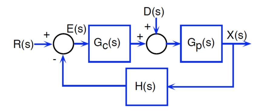
$$G_{cl}(s) = \frac{X(s)}{R(s)} = \frac{G_{c}(s)G_{p}(s)}{1 + G_{c}(s)G_{p}(s)H(s)}$$
