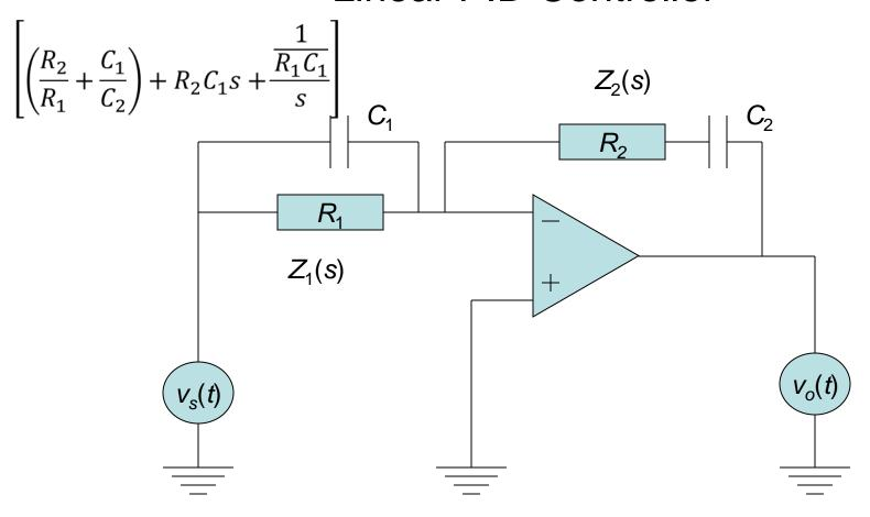
$$G(s) = \frac{V_o(s)}{V_S(s)} = -\frac{(R_1C_1s+1)(R_2C_2s+1)}{R_1C_2s} = \frac{R_2C_1s^2 + \frac{R_1C_1 + R_2C_2}{R_1C_2}s + \frac{1}{R_1C_2}}{s}$$
