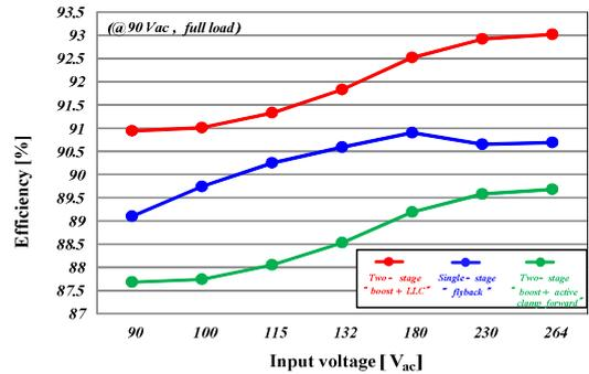
Fig. 17 Efficiency at 90 ~ 264 V<sub>ac</sub> input voltage
