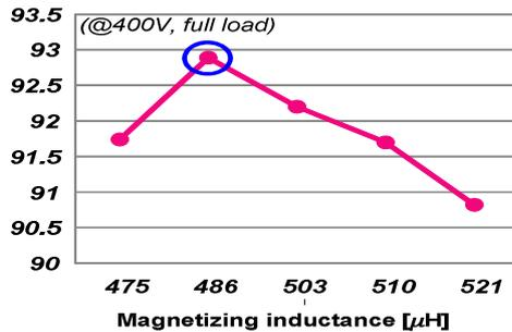
Fig. 12 Efficiency according to magnetizing inductance
