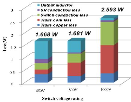
Fig. 11 Loss analysis according to different switch voltage rating
