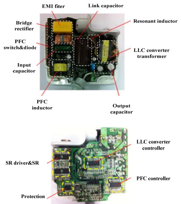
Fig. 18 Boost PFC + LLC DC-DC converter in conventional adapter case
