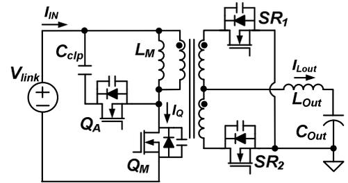
Fig. 5 Active clamp forward converter
