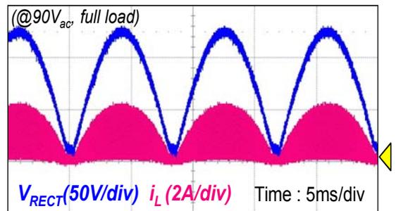
Fig. 10 Input voltage & current waveforms of boost PFC
