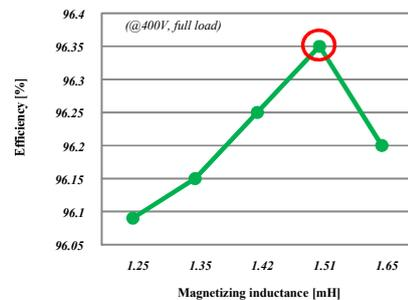
Fig. 14 Efficiency according to magnetizing inductance
