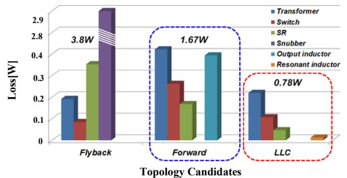
Fig. 7 Loss analysis of three DC-DC converters
