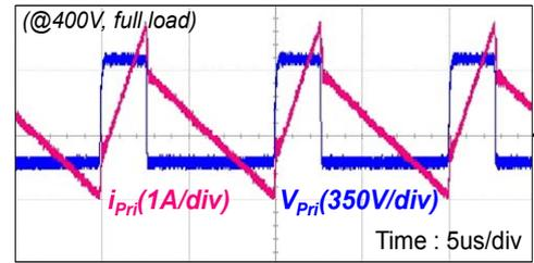
Fig. 13 Primary transformer voltage and current waveforms
