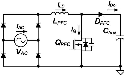
Fig. 3 Boost PFC converter
