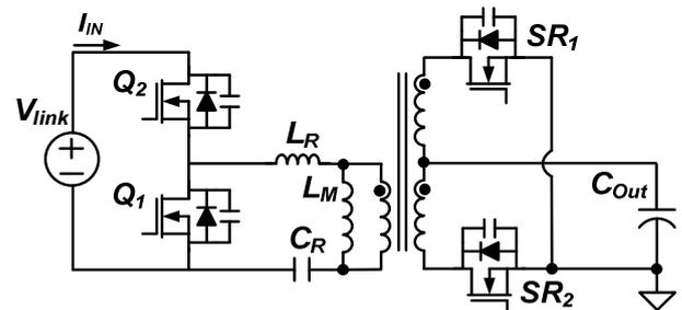
Fig. 6 LLC resonant converter
