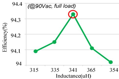
Fig. 8 Efficiency according to inductance value
