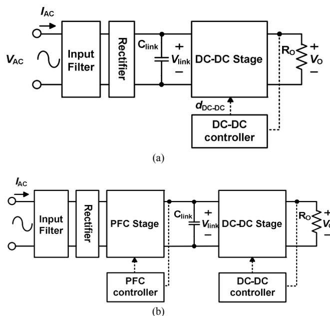
Fig. 1 (a) Conventional single-stage AC-DC converter structure
