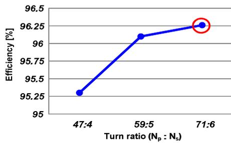
Fig. 15 Efficiency according to turn ratio
