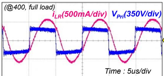
Fig. 16 Primary transformer voltage and resonant inductor current waveforms
