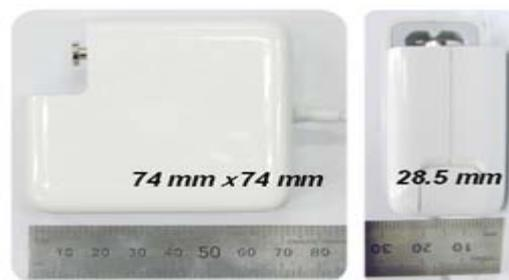
Fig. 2 Conventional single-stage AC-DC adapter case
